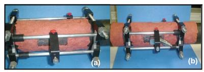
Figure 3-32: Clearing DMP-3 from the Transducer Location (a) and Installing the Transducers(b)
